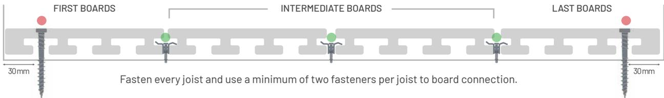
**Note:** Pre-drilling may be required when top fixing.
