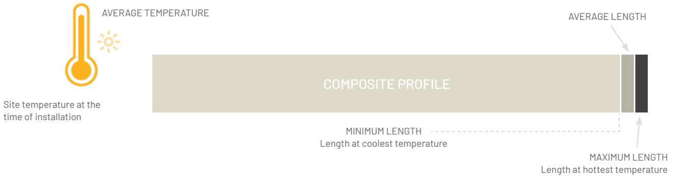
If the site is hotter than the expected average temperature, then the boards are expected to contract when the temperature drops to the average and the installed gap must be adjusted narrower accordingly.
