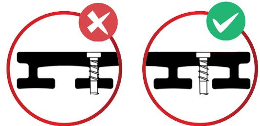
Avoid driving the top fixing screws through the web of the profile shape, this would cause cracking.
