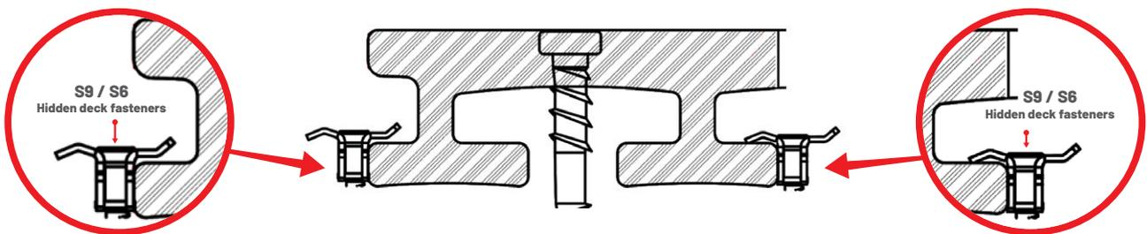
The I-Series board can be ripped but is limited to specific widths that allow the cuts to line up with the outer edge of the second or third foot to mimic the ends of the profile.
