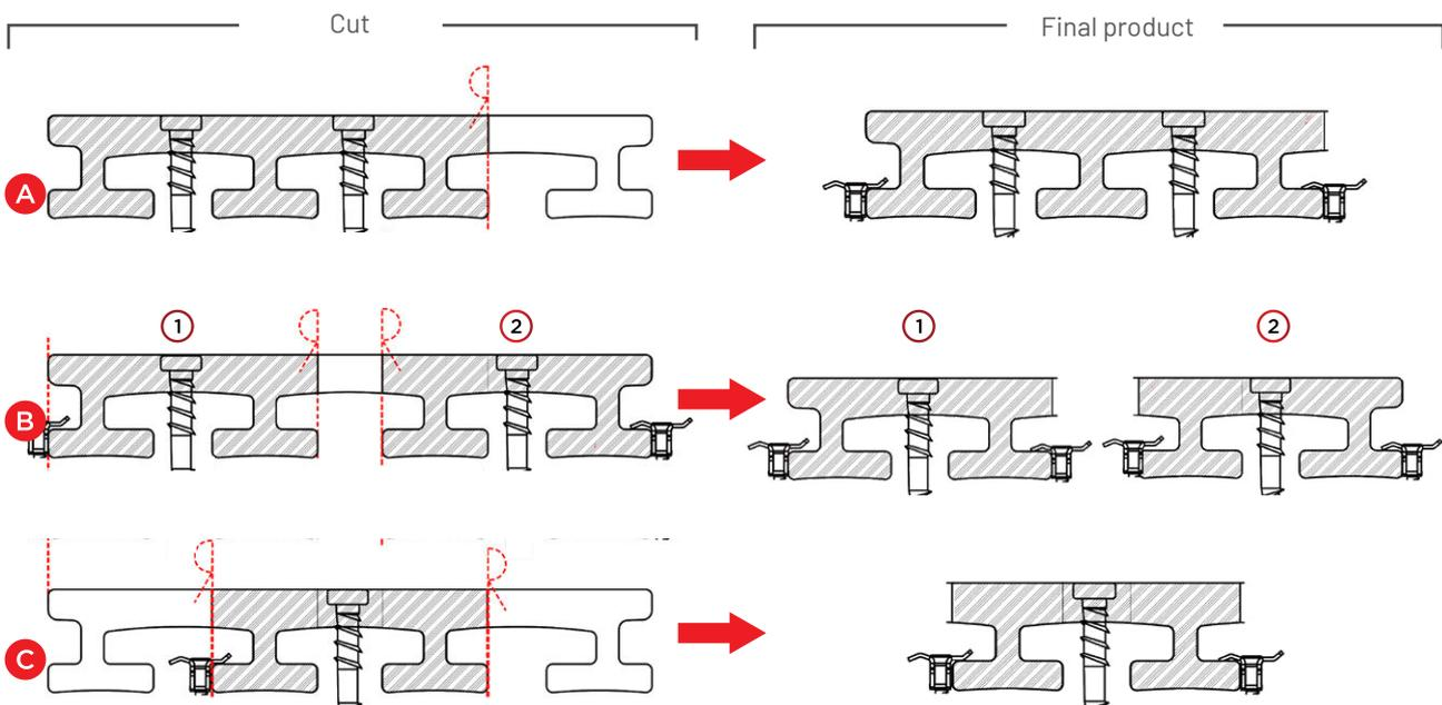
If the longitudinal profile of the ripped board is to be visible, it is good practice to install the board so that the cut face is turned inwards and the opposite face is exposed. However, in scenarios such as this, one should be able to extend the project area so that the final board can be a full board.
